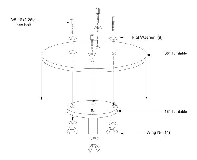
IN ORDER TO USE THE 36" TURNTABLE, IT MUST BE BOLTED TO THE 18" TURNTABLE AS SHOWN ABOVE IN FOUR PLACES, USING THE (4)3/8-16 X 2.25 LG. HEX BOLT, (8)3/8" SAE WASHERS AND (4) 3/8" WING NUTS.
